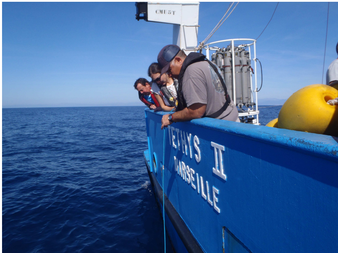
Measurement of the water transparency with the Secchi disk at the BOUSSOLE site from the deck of the R/V Téthys II .
